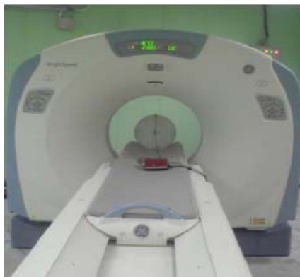
Fig. 2 Experimental setup for Dose measurement using the Barracuda dosimetry system
